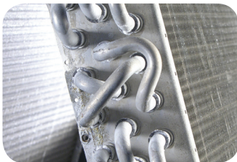
Aluminum tube and tube sheet after 500 hours in a controlled corrosive environment.
